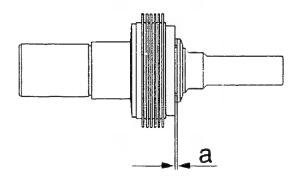
CHECKING AND REPAIRING COMPONENTS Checking multi-plate clutch Check overrunning torque of clutch. Clamp armature with clutch fitted in clamping support. Insert pinion in drive spindle. Check overrunning torque of multiplate clutch with torquemeter in non-friction direction. Torquemeter: 0 986 617 206 Overrunning torque: 0,2...0,4 Nm
